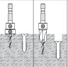
Packaged with grub screw for replacing drill and adjusting the depth stop
